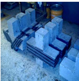
b) specimens after applied CFRP strips
